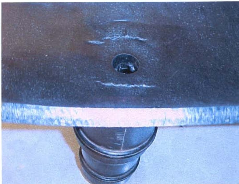
Pipe failure after 4815 h of pressure testing at +80°C, 4.6 MPa/5.7 bar. Standard requirement: Test time \geq 165 h
